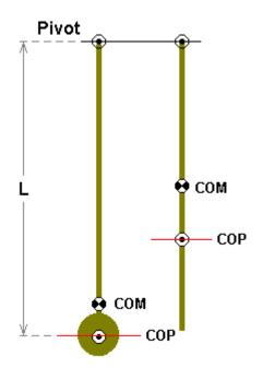
But as we've already observed, a tapered rod has a percussion point, relative to the heavy end, that's much less than a uniform rod. So our pendulum ends up with a much faster period, and a much shorter axis to percussion point distance, as shown in the following illustration. The question becomes how to keep from adding mass way down, which would be hard to swing, while still slowing down the frequency of the pendulum.
