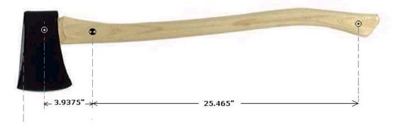
The axe is a Collins Commander, a 3 <sup>1</sup>/<sub>2</sub>-lb model, which weighs 4-lbs, 10.5oz. The 3<sup>1</sup>/<sub>2</sub>-lb description is a measure of head weight.
