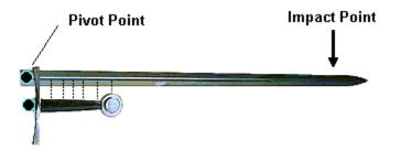
You might have a flash of inspiration and go for a giant pommel, but this doesn't work. It shifts the axis of rotation so close to the pommel that the sword can't be swung. Even just going with an overly large pommel just moves the percussion point out so far that the sword loses its tendency to realign itself during a swing.
