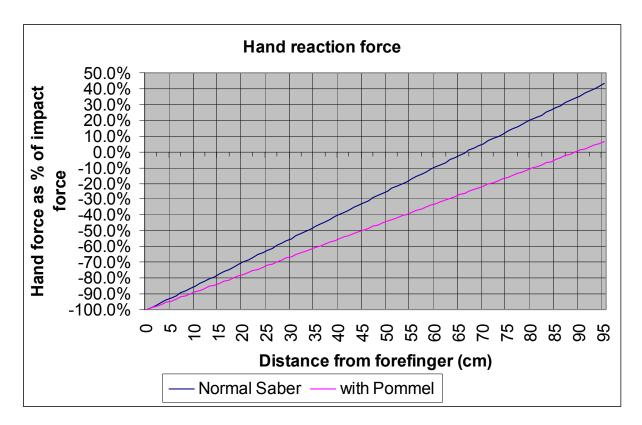
Just for completeness, here is the hand force verses impact force for the Austrian saber after adding a 341g pommel. Notice that for cuts near the tip the hand shock is much less than the unmodified saber.
