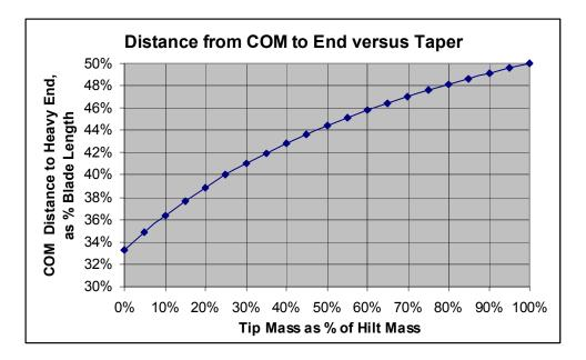
We also have the center of mass moving away from the heavy end, as the amount of taper decreases, as shown in this chart. If you have a bare blade, its balance point can give a fair indication of how much mass tapering it has. This mass tapering can be easier to feel, than to see. But this chart will help in evaluating what kind of blade you might have in your hand. It ignores the effect of the tang, which will be addresses in a different section on tang thickness and strength.
