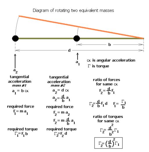
Here, for a given angular acceleration  $\alpha$  (alpha), the tangential acceleration, a, of each mass, is determined by the distance of the mass from the axis of rotation. The ratio of the linear acceleration of the second mass, compared to the first, is the same as the second masses distance from the axis compared to the first masses (d/b). But it also takes more
