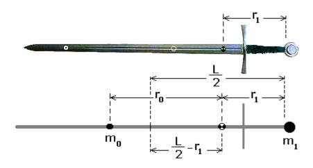
First, calculate the moment of inertia of the rod about the desired center of mass location. The distance from the pommel end of the rod to the sword's center of mass is just  $r_1$ , as shown, while the distance to the center of the rod is  $\frac{L}{2}$ , where L is 4 feet, or 1.219 meters. So we want to know the moment of inertia of the rod when we shift to distance of  $\frac{L}{2} - r_1$ . Using the
