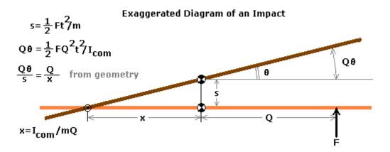
Here's an exaggerated diagram of an impact where  $\theta$  is made large for clarity. The light brown stick is the initial position, the dark brown stick the position at the end of the impact event. The impact consists of the force F applied at distance Q from the center of mass (the little round symbol in the center of the stick). The center of mass accelerates away and travels the small
