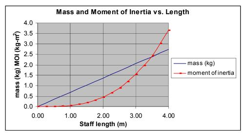
This chart shows how increasing length increases the mass and moment of inertia about the center of mass of a 1.5-inch (38mm) diameter staff, made of ash or white oak. Note how fast the moment of inertia builds up, making a long staff very unwieldy. For a given torque applied by your arms, the staff's maneuvering accelerations are inversely proportional to the moment of inertia. So the maximum attainable rotational acceleration is plummeting as length increases.
