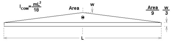
This staff is midway between a non-tapered version, with  $I_{COM} = \frac{mL^2}{12}$ , and the fully tapered
