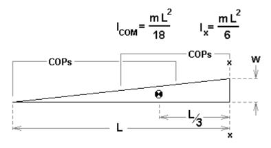
Recall that the moment of inertia of a uniform stick was  $I_{COM} = \frac{mL^2}{12}$ . With uniform taper we
